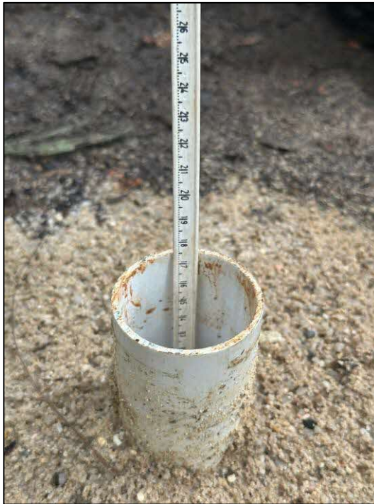
Figure 5.9. Example of groundwater level survey being conducted
